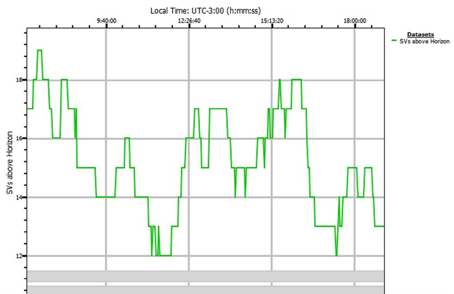
FIGURE 18 Prediction of satellites above horizon on 19 September 2017 (experiment day 7) at UFSCar reference point
